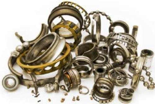
This is a selection of failed or damaged bearings, many resulting from high contamination levels.
